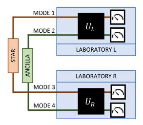
FIG. 7. Scheme of generalized Gottesman *et al.* protocol. The ancilla and measurements are kept the same as in the original proposal. We restrict this analysis to the local operations  $U_L$  and  $U_R$ .
