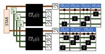
FIG. 3. Scheme of the modified version of Khabiboulline's protocol for N=7 time bins.  $\overline{\text{CZ}}_k(i)$  indicates a sequence of controlled phase gates with k target qubits (ancilla) corresponding to the ith time bin.
